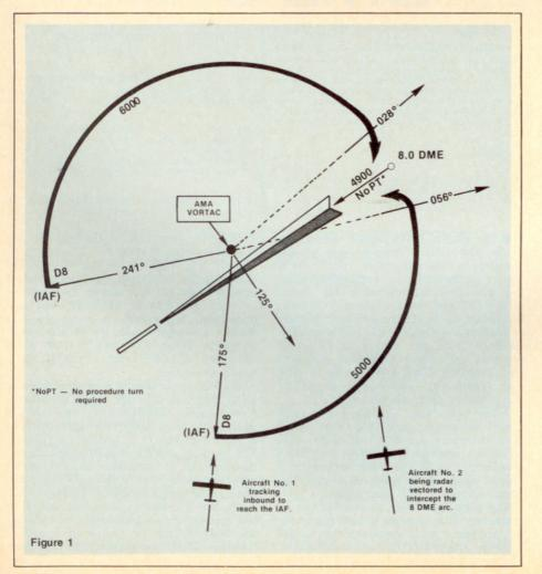
It is also possible that a pilot might be radar-vectored to intercept the DME arc at a point other than at an IAF. Aircraft No. 2 in the diagram has been cleared to maintain a given heading and intercept the 8 DME arc at which point he should begin orbiting the VORTAC as shown on the approach plate.
